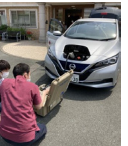
Deployment of emergency power supply
