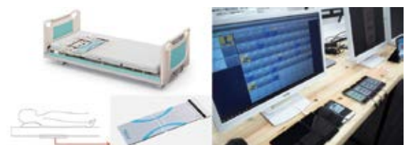
Sensors measure body movements to ascertain the condition of a bed's occupant while asleep.
