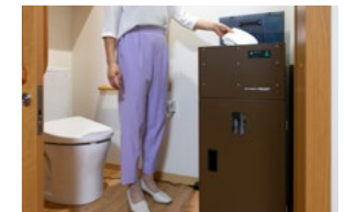
"wrapponn-PACKET," a diaper collection box with an automatic wrapping mechanism
