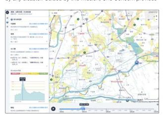
Damage prediction system for flood
